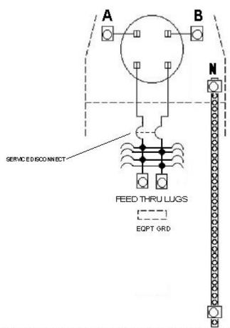
Short Circuit Current Rating (Watthour Meter not included in short circuit current rating) This panelboard has a maximum short circuit rating of 22,000 RMS symmetrical amperes, 240 volts maximum with Siemens type EQ9685 main breaker installed. Any branch circuit breaker installed, replaced or added in this panelboard must be manufactured by Siemens and must be of the types listed below.
