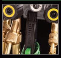
Attach K-style clamp to an easily accessible spot on the hilmor manifold.
